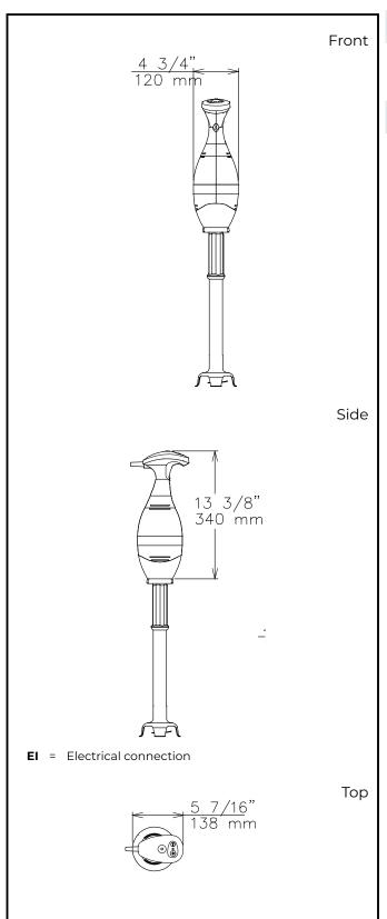
Electric Supply voltage: 110-120 V/1 ph/50/60 Hz **Total Watts:** 0.75 kW Plug type: USA NEMA 5-15P Key Information: External dimensions, Width: 5 7/16" (138 mm) External dimensions, 4 3/4" (120 mm) Depth: External dimensions, 38 " (965 mm) Height: **Shipping width:** 11 7/16" (290 mm) Shipping depth: 27 3/16" (690 mm) Shipping height: 7 1/16" (180 mm) **Shipping weight:** 12 lbs (5.6 kg)
